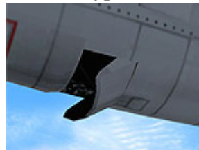
Engine Oil cooler flaps(4) VC
