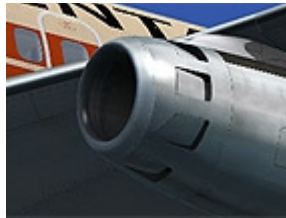
Engine intake flaps (14)
