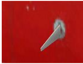
Angle of attack sensors (2)
